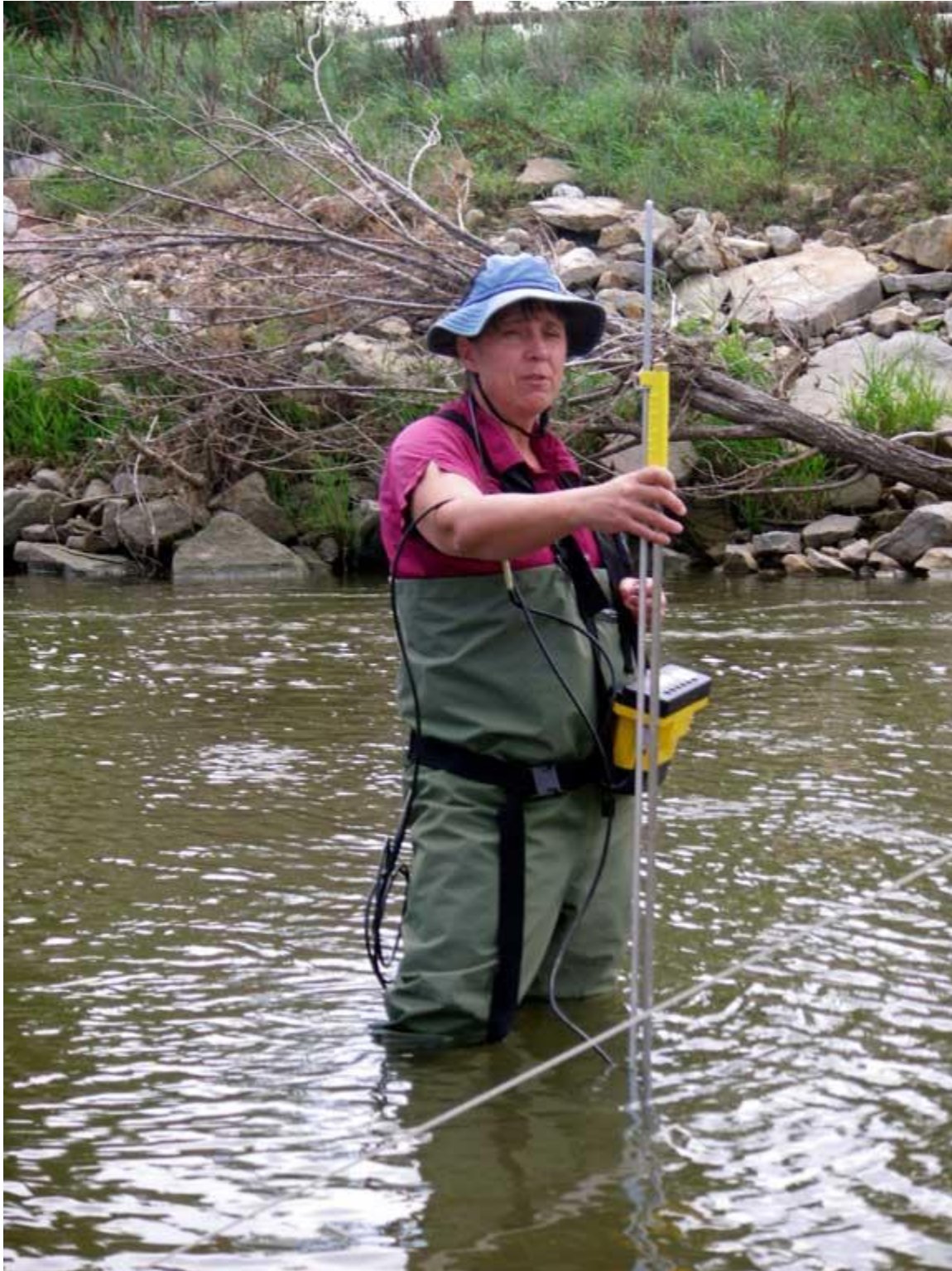
Figure 2. Water and Earth Technologies' Kate Malers measuring water velocity and depth across the channel at the County Road 13 site. Below the water's surface is a device that measures the velocity and marks on the rod measure depth.
